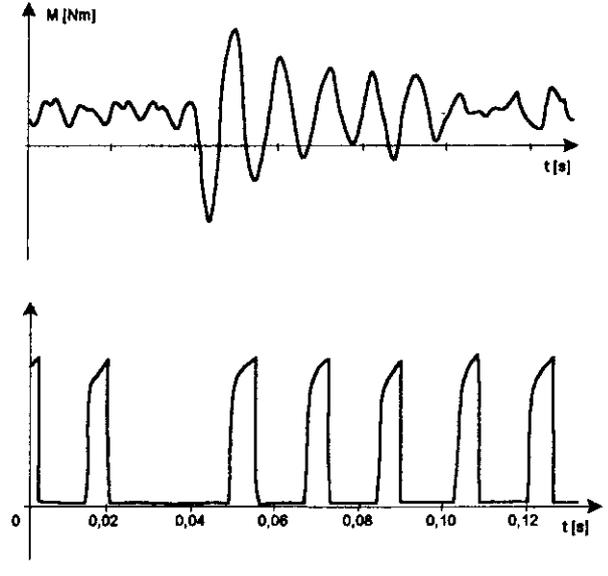
Figure 12. Torque and ignition signals for 3500 rpm, throttle 100%, 1 misfire [6]
