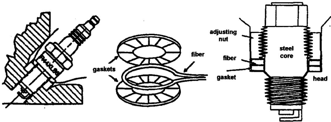
Figure 19. Fiber optic sensor integrated with the gasket [18]
