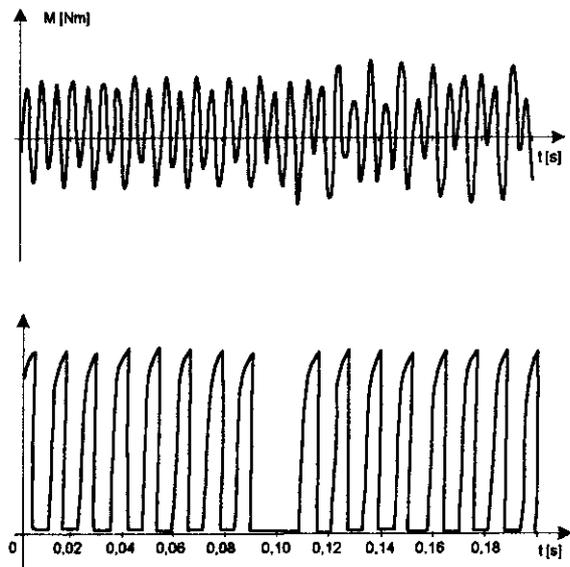
Figure 13. Torque and ignition signals for 5000 rpm, throttle 50%, 1 misfire [6]
