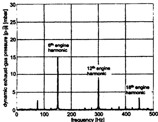
Figure 5 Amplitude spectrum of the exhaust-gas pressure measured in the catalyst mixing tube without misfires, engine speed 3000 rpm, mid-load [5]
