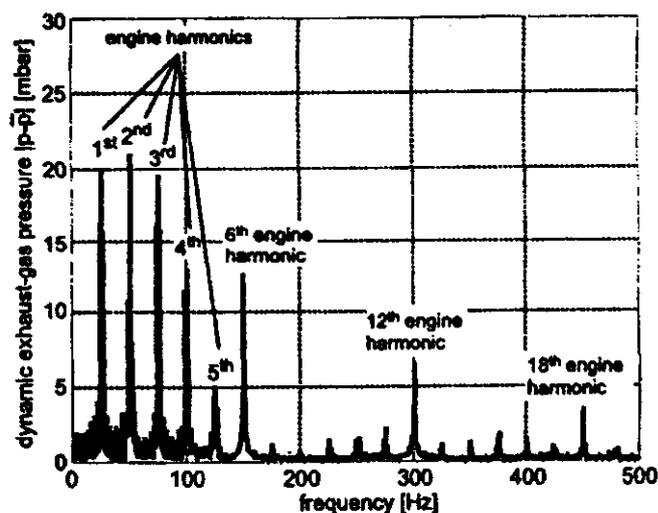
Figure 6 Amplitude spectrum of the exhaust-gas pressure measured in the catalyst mixing tube with misfires in cylinder 2, engine speed 3000 rpm, mid-load) [5]
