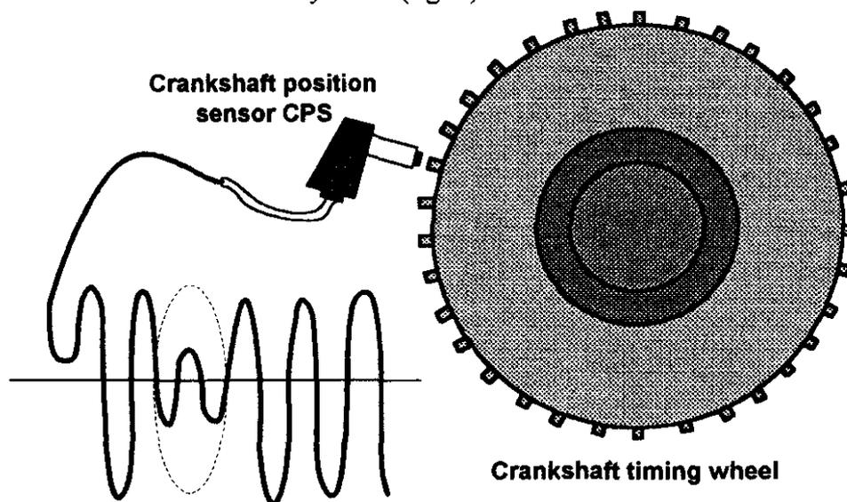
Figure 1 Recognition system for misfire detection on the basis of changes in crankshaft speed [15]
