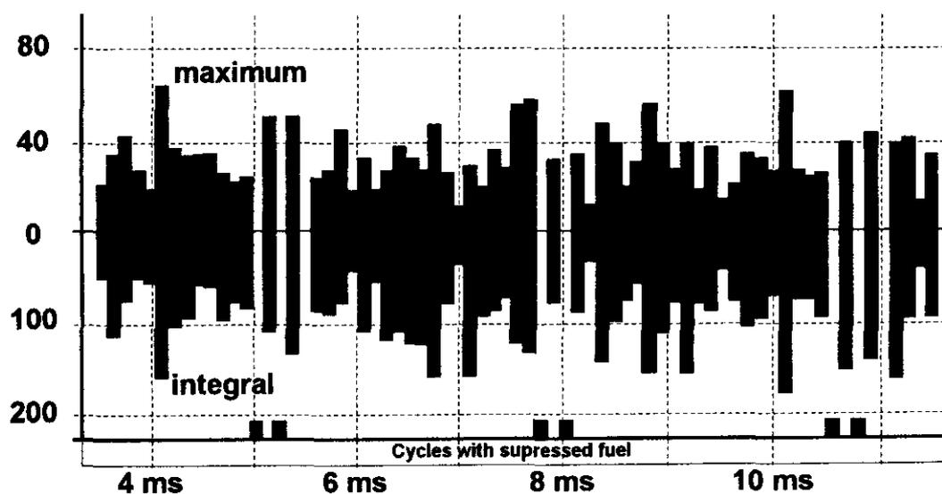
Figure 9 Sequence of calculated features in dependence of the time. Herein the results of 2 cylinders are alternately multiplexed [10]
