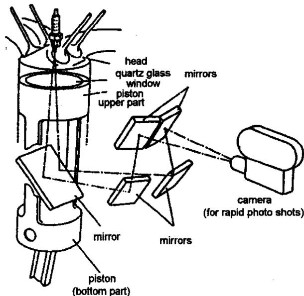
*Figure 16. General overview of Stereography Method for Gas Flow Investigation [16]*
