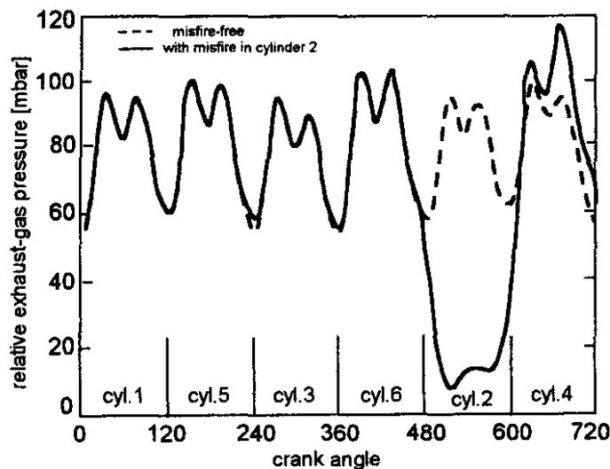
Figure 4 Comparison of the relative exhaust-gas pressure measured in the catalyst mixing tube without misfires and with a misfire in cylinder 2, engine speed 3000rpm, mid-load [6]
